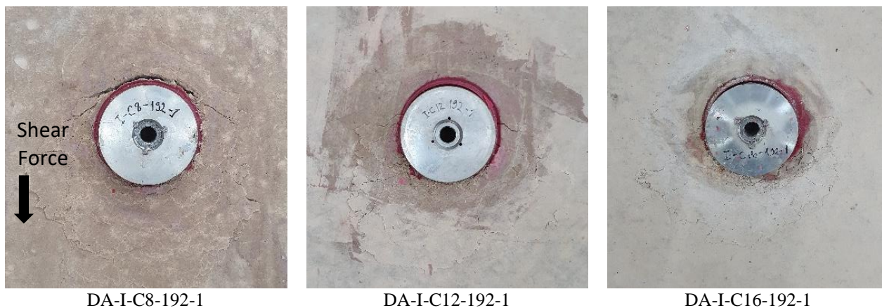
Fig. 7 - Typical failure condition after the shear test
